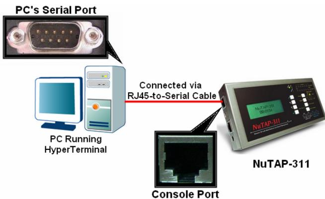
By connecting NuTAP-311's **Console Port** to PC's **Serial Port** via **RJ45-to-Serial** cable, you can configure/view NuTAP-311's settings with **HyperTerminal** softwares installed on your PC.
