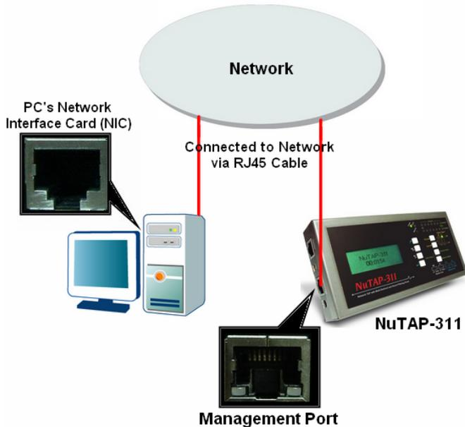
By connecting NuTAP-311 and PC to the same network, you can configure/view NuTAP-311's settings with the web browser installed on your PC.
