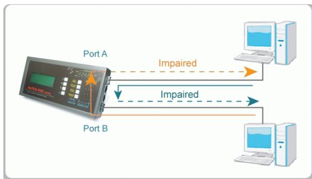
Data streams both way that flow through this machine is impaired
