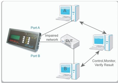
In the illustration figure above, a good DUT should have correct reaction on impaired network and the computer A and B should get all data correctly. In addition, If A and B get all data correctly, does it fit the performance or recovery action required.
