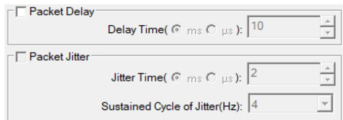
NuTEA-551 can emulate Packet Delay and Packet Jitter with its utility software, as shown in the figure above. The Delay/Jitter Time can be set in milliseconds (ms) or microseconds ( $\mu$ s).
