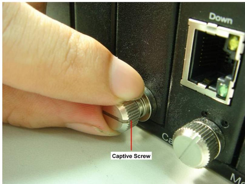
Lock the Captive Screw into the MCS-2160 to fix the Bracket into MCS-2160.
