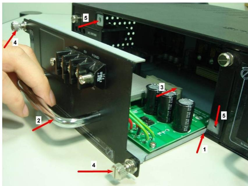
Installing a XCP-DC-300 into MCS-2160 is quite simple. First of all, attach the Power Module into the respective slot of MCS-2160 and push the handle of the Power Module into the slot. After the Bracket of the Power Module reaches the MCS-2160, lock the captive screw into MCS-2160 as shown by arrows 4 and 5.
