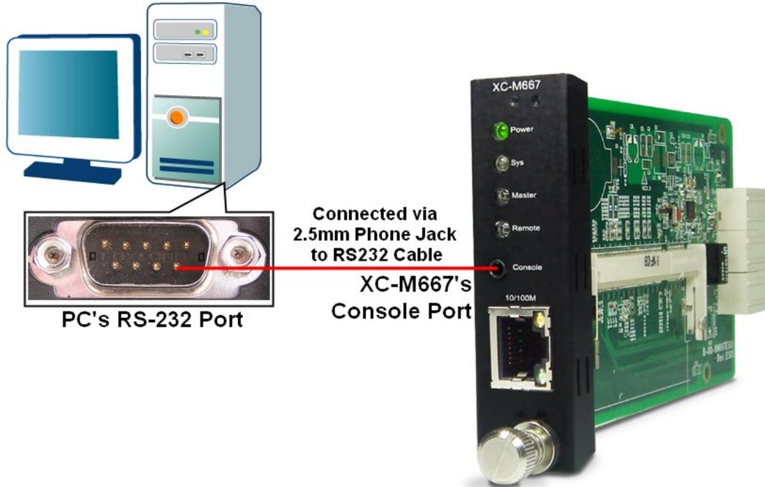
MCS-2160 allows users to make system configurations and view test statistics/system information with **HyperTerminal**. To access MCS-2160 via **HyperTerminal**, you have to connect XC-M667's **Console Port** with **PC's RS-232 Port** via a 2.5mm Phone Jack to RS-232 cable as shown in the figure above.
