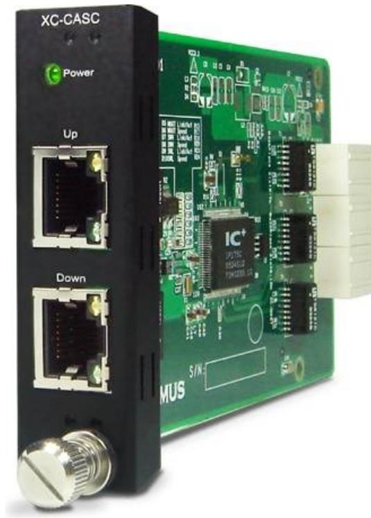
The **XC-CASC** comes with your MCS-2160 chassis, and shall be installed on the **Casc** slot located on the right side of MCS-2160 chassis (next to **XC-M667** module card). This module card allows you to cascade multiple MCS-2160 chassis.
