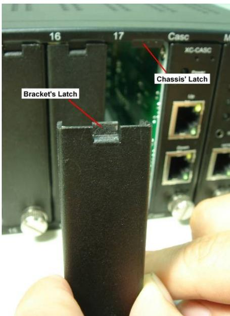
Attach the Bracket's Latch on the internal face of Chassis' Latch.
