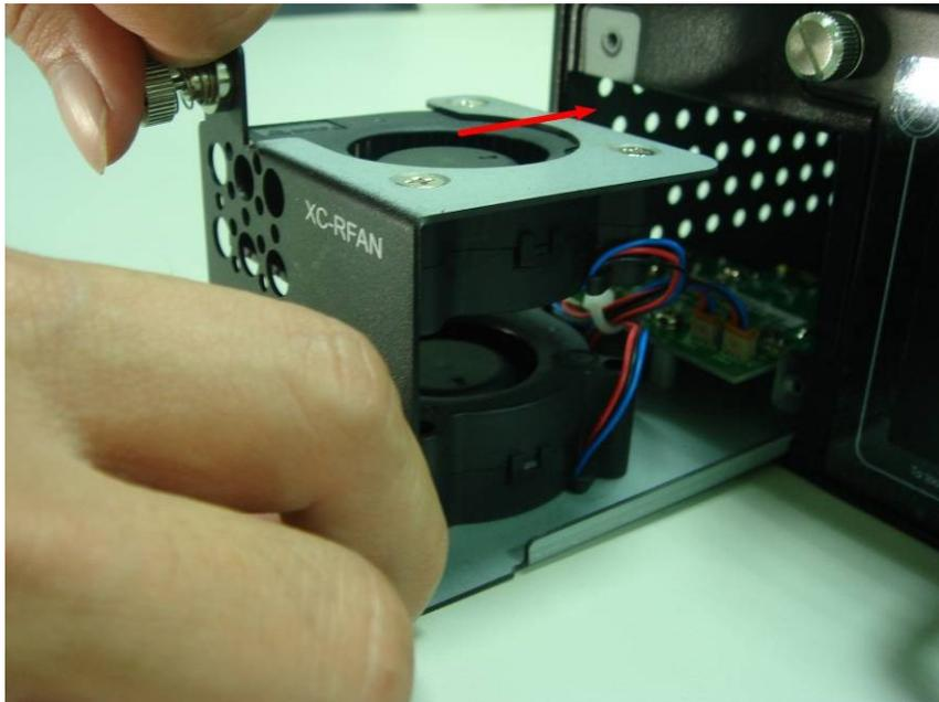
Installing the XC-RFAN is quite simple, just attach the XC-RFAN into the respective slot of MCS-2160, and push it into the slot. After the Bracket of the XC-RFAN reaches the MCS-2160, lock the captive screw into MCS-2160.
