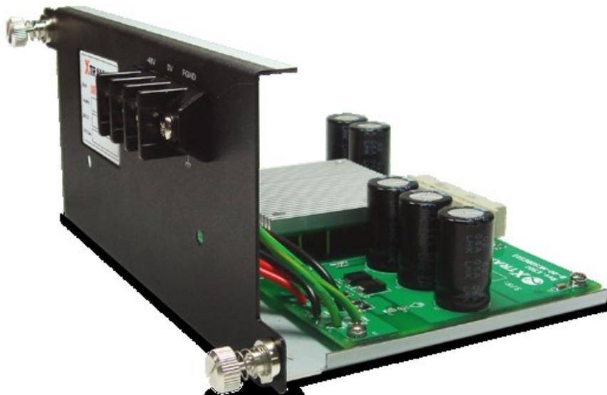
The Power Jack of XCP-DC-300 is 3 Terminal Connectors: -48V, OV, FGND. The Terminal Connector -48V and OV have a screw to fix an external power source cable. The FGND also has a screw, but this screw should be fixed with an external cable connected to the ground.
