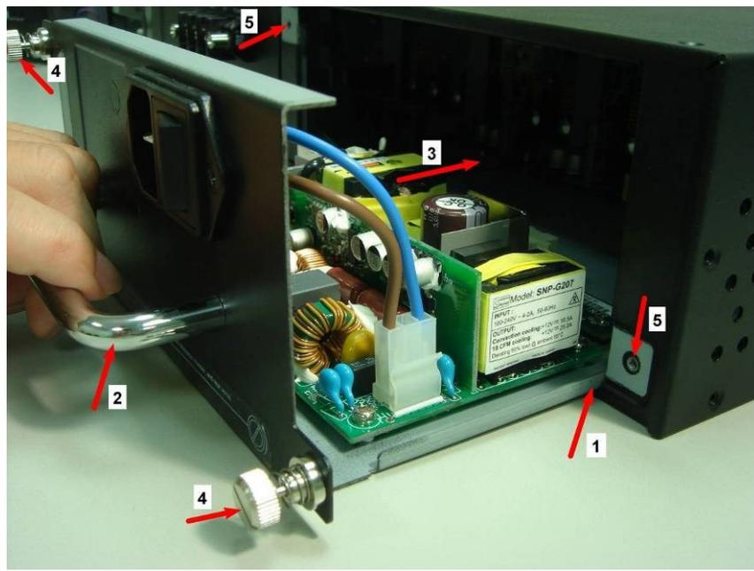
Installing a XCP-AC-300 into MCS-2160 is quite simple. First of all, attach the Power Module into the respective slot of MCS-2160 and push the handle of the Power Module into the slot. After the Bracket of the Power Module reaches the MCS-2160, lock the captive screw into MCS-2160 as shown by arrows 4 and 5.
