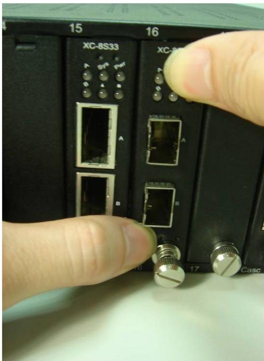
Please, make sure if the Media Converter Module Card is well fixed into MCS-2160 by pushing the bracket of the Module Card into MCS-2160.
