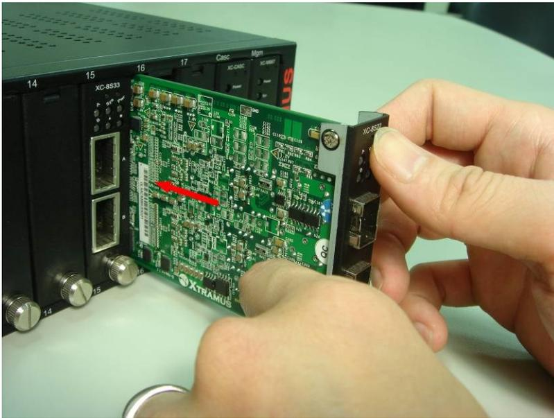
Aim the border side of a Media converter Module Card with the MCS-2160 internal slide road, and push this Module Card into MCS-2160.
