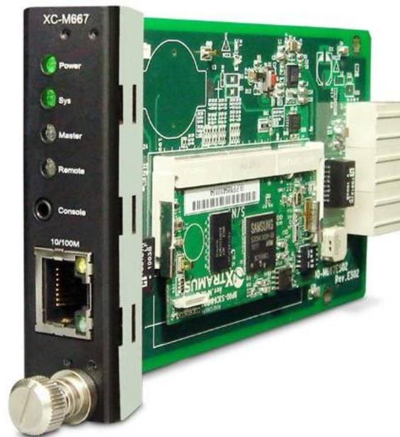
The **XC-M667** comes with your MCS-2160 chassis, and shall be installed on the **Mgm** slot located on the far right side of MCS-2160 chassis. This module card allows you to manage MCS-2160 chassis via management webpage.
