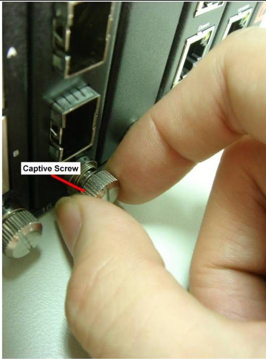
Lock the Captive Screw into the MCS-2160 to fix the Module Card into MCS-2160.
