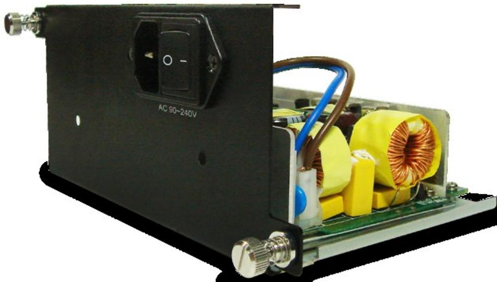
The Power Jack of XCP-AC-300 is Male IEC 320 Receptable. To activate XCP-AC-300 & XCP-AC-100, just turn on/off the O/I button after connecting a power source cable in Male IEC 320 Receptable.
