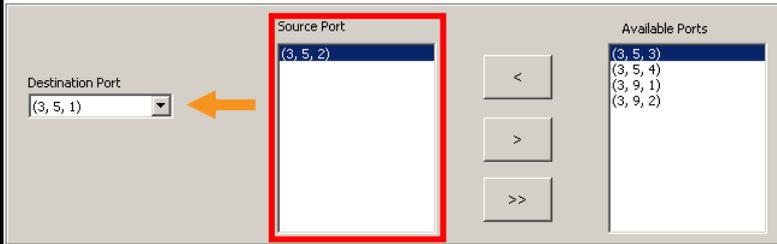
4. The port you've selected will be added to the **Source Port** field. You can remove one source port by clicking the **>** button, or remove all source ports by clicking the **>>** button.
