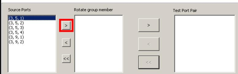
2. Click the **>** button to add the port you've selected in step 1. The ports you've added will be shown in the **Rotate Group Member** field. You can remove one port by clicking the **<** button, or remove all ports by clicking the **<<** button.
