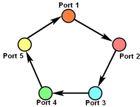
In **Rotate** test mode, packets will be sent from port to port in a loop while the last port will be connected to the first port, as shown in the figure above.
