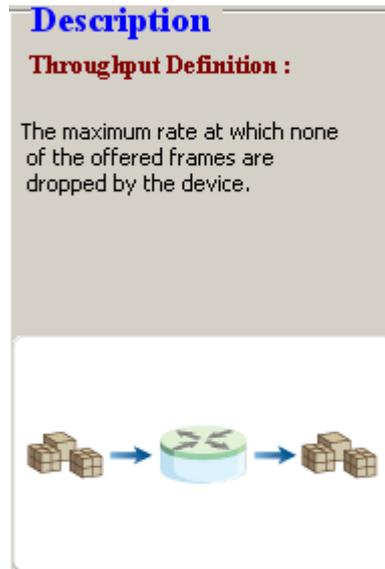
The **Description** displays brief descriptions and figures regarding to **Throughput, Latency, Packet Loss,** and **Back to Back** tests.
