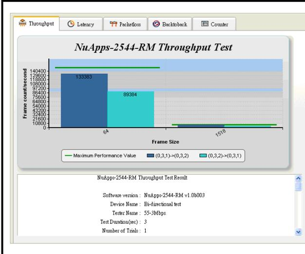
The **Report** on the **System Info/Configuration List** allows you to view test results, charts, and statistics on the **Main Display Screen** located on the right side of NuApps-2544-RM's main window.
