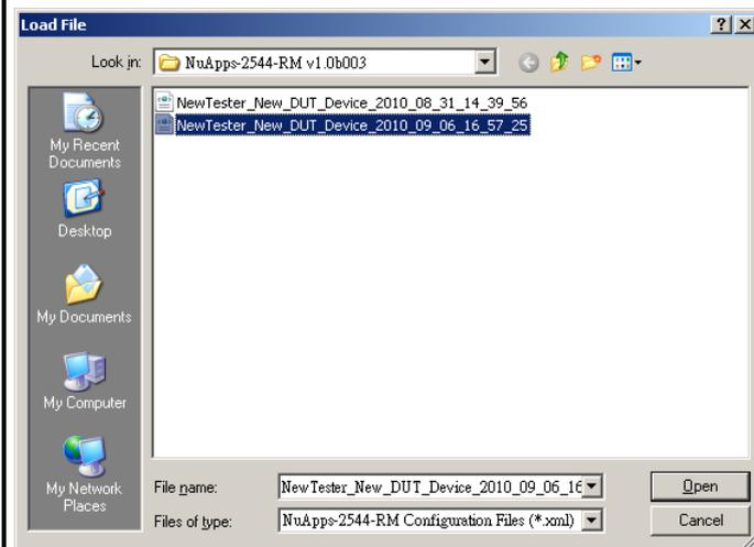
If you have a previously saved configuration file stored in your PC, you can load it and apply all the setting you’ve made by choosing “**Open an Existing Configuration**” from the **Select Config** pop-up window.
