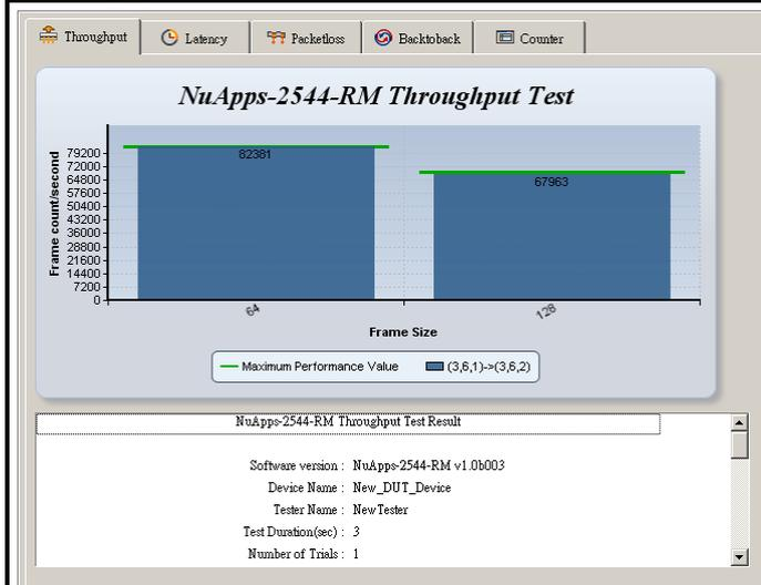
This chart uses **Frame Count per Second** as X-Axis, and **Frame Size** as Y-Axis to show DUT's throughput performance.
