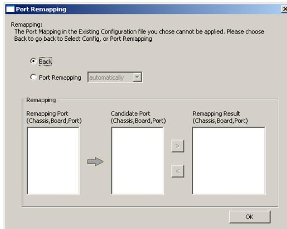
If the port mapping contained in the configuration file you've loaded from your PC does not match NuStreams-2000i/600i's current port mapping, a **Port Remapping** window will pop up and guides you through port remapping process.
