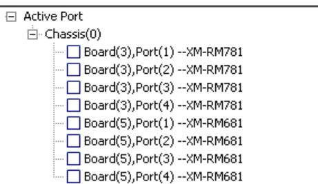
All the module cards, along with their Active Ports are listed here in this field. You can fold/unfold the tree style tab by clicking / icons. Also, you can check/uncheck the port by clicking  icon.
