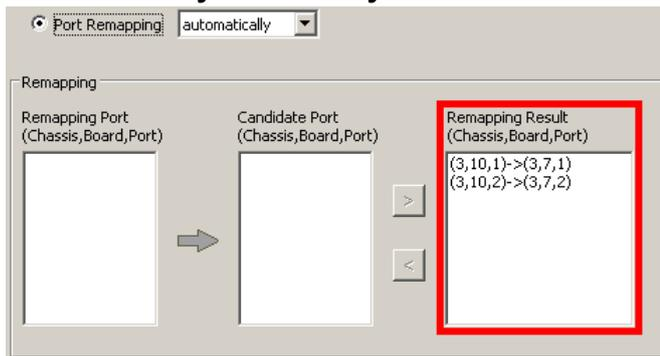
If you choose **automatically** from the **Port Remapping** scroll-down menu, NuApps-2544-RM will make the proper port remapping automatically.
