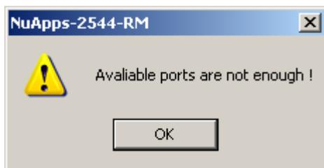
If the module card information contained in the configuration file you’ve loaded from your PC has more module cards than your current amount of module cards, a warning message will pop up, showing that “**Available ports are not enough**”.
