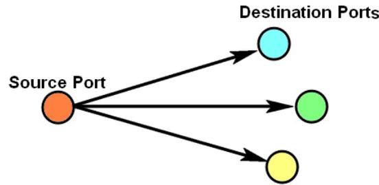
In **One to Many** test mode, packets will be sent from one source port to multiple destination ports as shown in the figure above.
