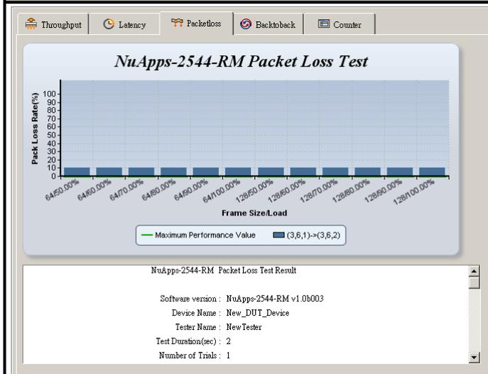
This chart uses **Packet Loss Rate (%)** as X-Axis, and **Frame Size/Load** as Y-Axis to show DUT's packet loss ratio.
