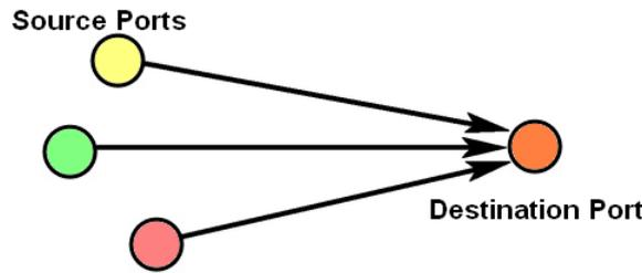
In **Many to One** test mode, packets will be sent from one destination port to multiple source ports as shown in the figure above.
