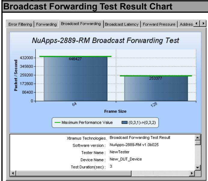
This chart uses **Packet/Second** as Y-Axis, and **Frame Size** as X-Axis to show DUT's Broadcast Forwarding performance.
