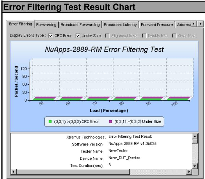
This chart uses **Packet/Second** as Y-Axis, and **Load (Percentage)** as X-Axis to show DUT's Error Filtering performance.
