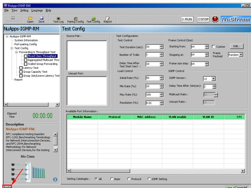
The **Status Bar** indicated by the arrow above shows the running status of NuApps-2889-RM. The running status includes: "Testing", "Performing testing", "Ready" and others.
