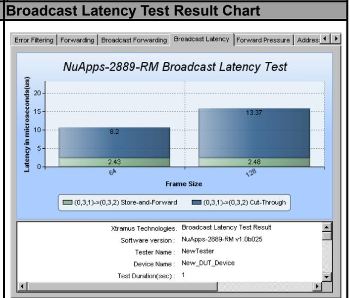
This chart uses **Latency in Microsecond (us)** as Y-Axis, and **Frame Size** as X-Axis to show DUT's Broadcast Latency test result.
