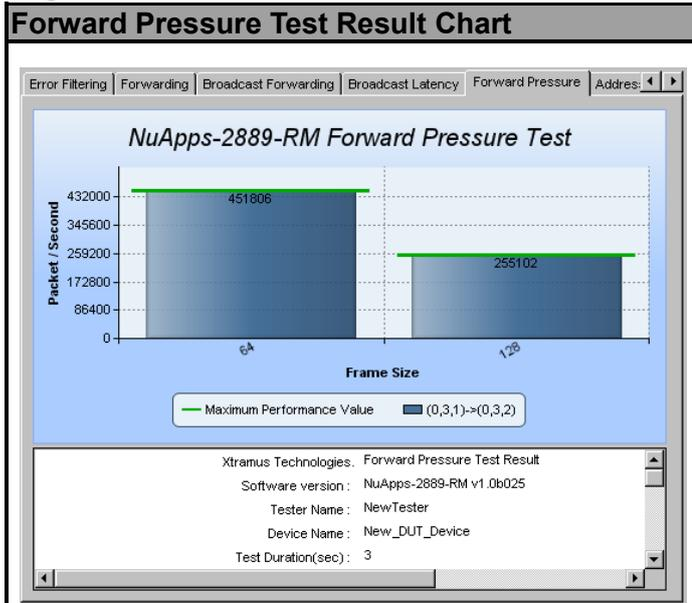
This chart uses **Packet/Second** as Y-Axis, and **Frame Size** as X-Axis to show DUT's Forward Pressure performance.
