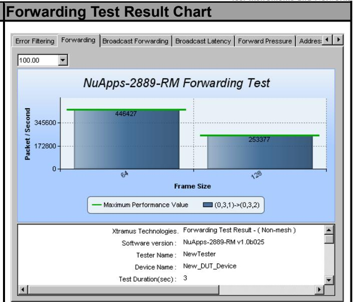
This chart uses **Packet/Second** as Y-Axis, and **Frame Size** as X-Axis to show DUT's Forwarding performance.
