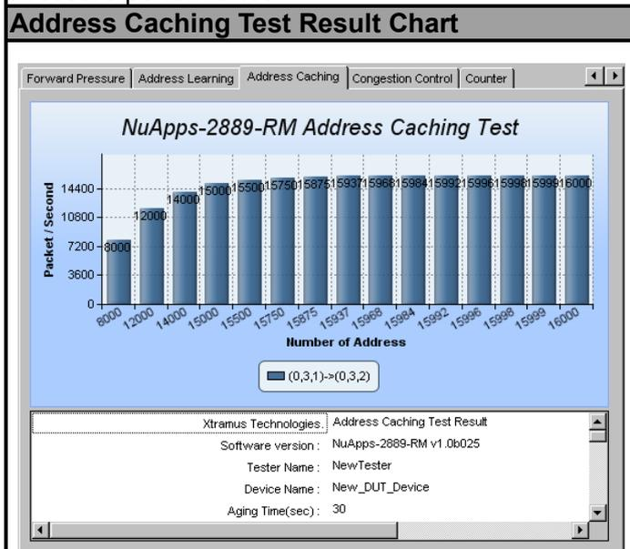
This chart uses **Packet/Second** as Y-Axis, and **Number of Address** as X-Axis to show DUT's Address Caching performance.
