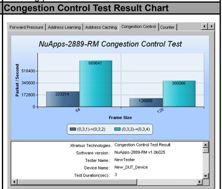
This chart uses **Packet/Second** as Y-Axis, and **Frame Size** as X-Axis to show DUT's Congestion Control test result.
