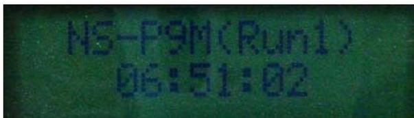
4. Connection established, and NuPAD's buzzer stops beeping. If NuPAD's buzzer keeps beeping and the connection between NuStreams-P9M and NuPAD can't be established, please power off both NuStreams-P9M and NuPAD, power them on, and try again.
