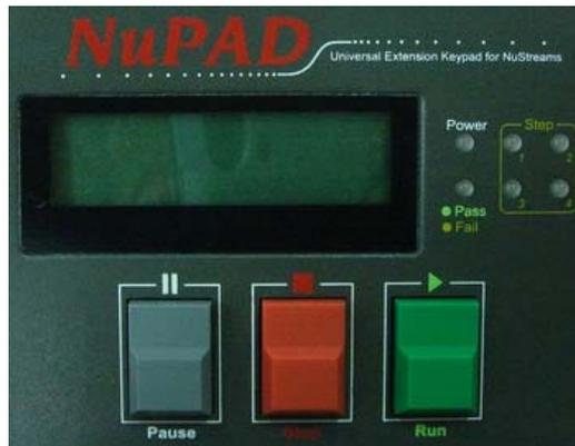
NuPAD has 3 buttons on its front panel: “|| **Pause**”, “■ **Stop**”, and “▶ **Run**”. After connecting NuPAD with NuStreams-P9M with Cat-5 cable, you can start/pause/stop DUT tests with these 3 buttons.
