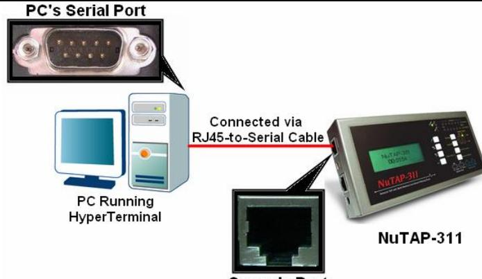
By connecting NuTAP-311's **Console Port** to **PC's Serial Port** via **RJ45-to-Serial cable**, you can configure/view NuTAP-311's settings with **HyperTerminal** softwares installed on your PC.
