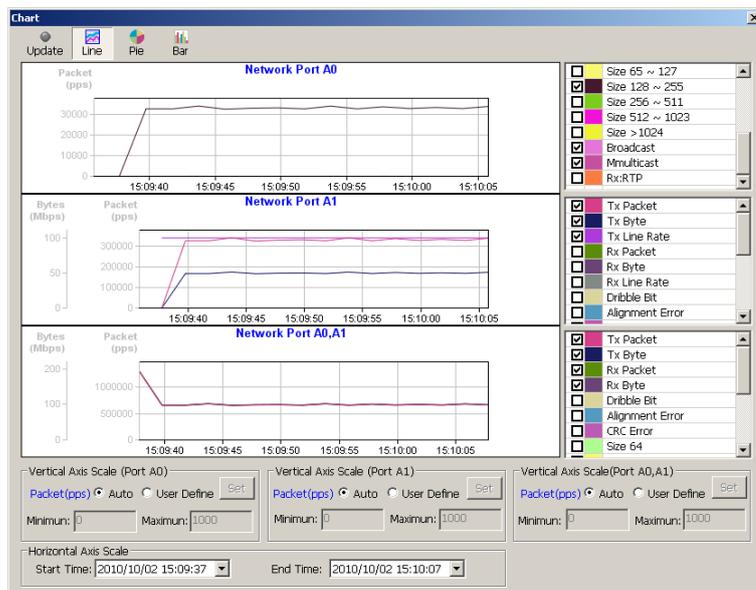
The **Line Mode** displays the statistics about the of packets flow through **Network Port A0**, **Network Port A1**, and **Network Port A0/A1**. To display the statistics as line on the chart, please click the check box of that statistics.
