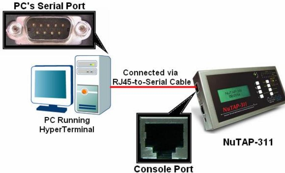
NuTAP-311 allows users to make system configurations, view test statistics/system information with **HyperTerminal**. To access NuTAP-311 via **HyperTerminal**, you have to connect NuTAP-311's **Console Port** with **PC's Serial Port** via an **RJ45-to-Serial cable** as shown in the figure above.
