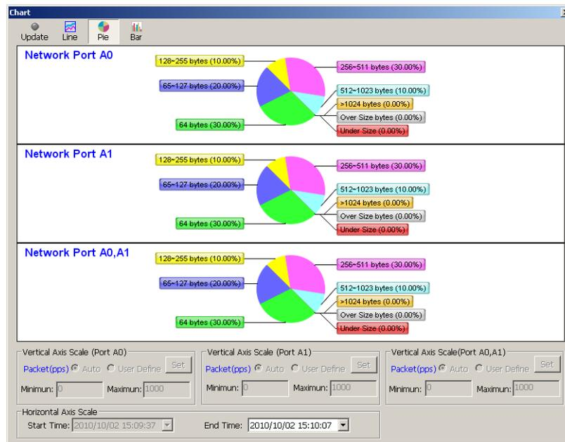
The **Pie Mode** displays the statistics regarding to the lengths of packets flow through **Network Port A0**, **Network Port A1**, and **Network Port A0/A1**. Packets are categorized into the following categories: **64 bytes**, **65~127 bytes**, **128~255 bytes**, **256~511 bytes**, **512~1023 bytes**, **>1024 bytes**, **Over Size byte**, and **Under Size**.
