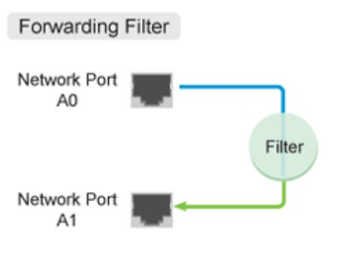
With **Forwarding Filter**, NuTAP-311 will transmit packets from Network Port A0 to A1 (or the other way around) that meet the criteria set in **Forwarding Filter** will be filtered out or through. The **Forwarding Filter** setting screen contains three tab-menus: **Protocol**, **SDFR** (Self-Discover Filtering Rules), and **Result**.
