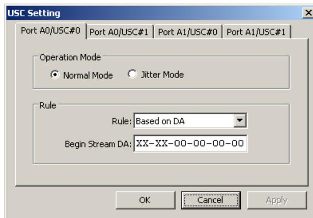
A **USC Setting** window will pop up if you click the **Setting** button, allowing you to set USC criteria for **Port A0/USC#0**, **Port A0/USC#1**, **Port A1/USC#0**, and **Port A1/USC#1**. To choose the Universal Stream Counter you would like to configure, please click the tab-menu on the upper part of the **USC Setting** window.
