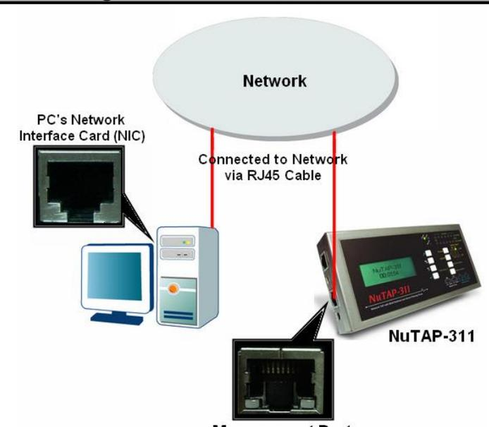
By connecting **NuTAP-311** and **PC** to the **same network**, you can configure/view NuTAP-311's settings with the web browser installed on your PC.
