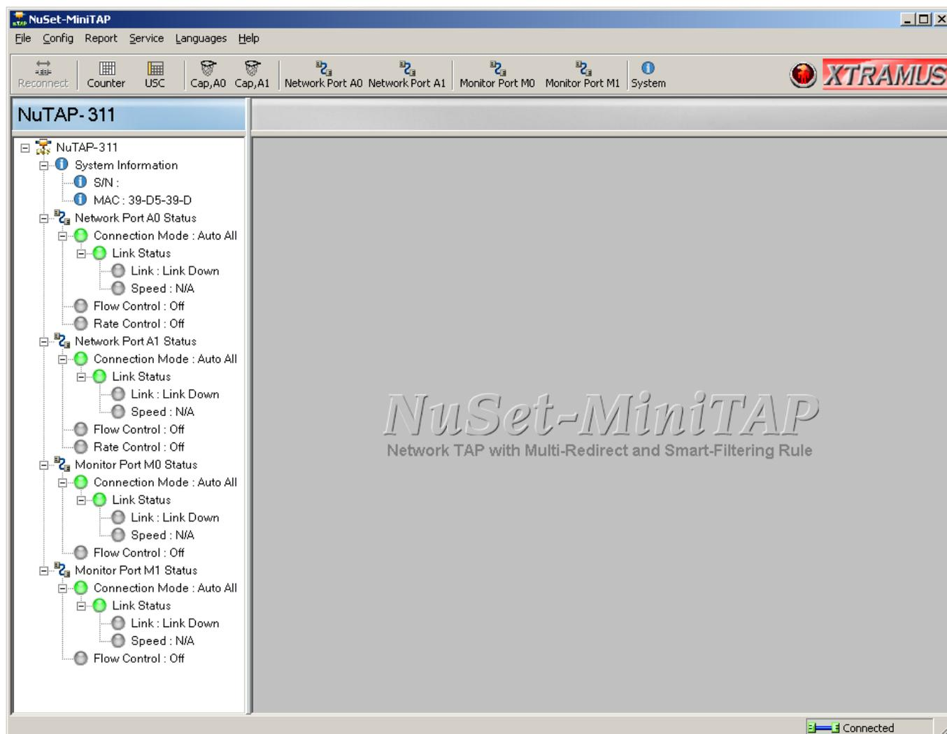
When NuTAP-311 is connected with PC via its **USB** cable, you can set test criteria, save/view testing logs, and upgrade NuTAP-311's firmware/FPGA with **NuSet-MiniTAP**.
