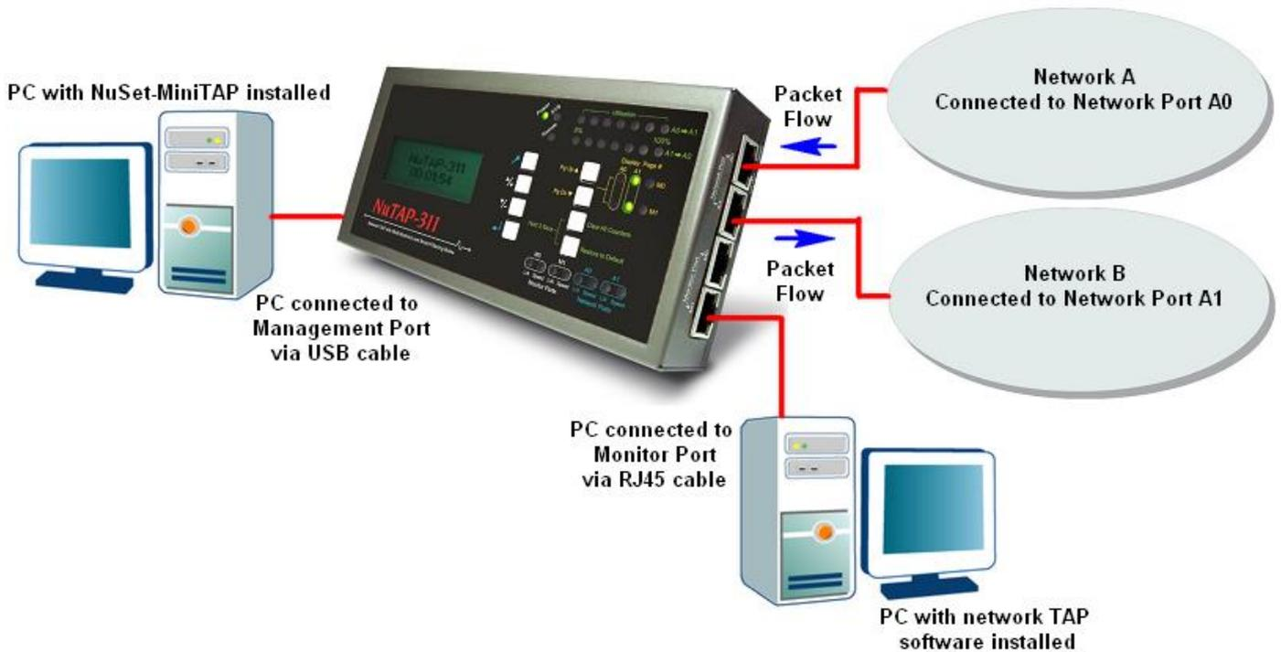
As the example shown in the figure above, NuTAP-311 allows you to perform network tapping. You can monitor/filter packets that meet the criteria by:
