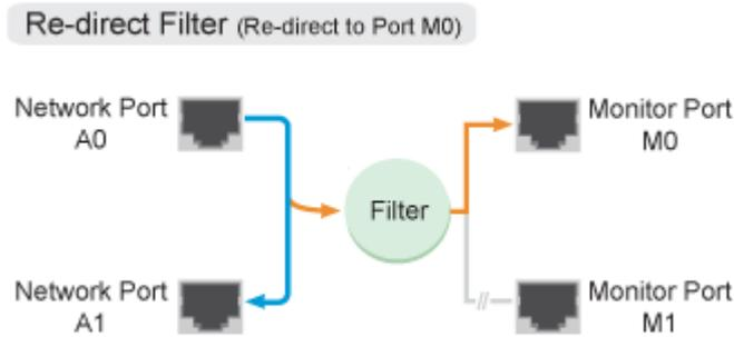
With **Re-Direct Filter**, transmitted packets from specific **Network Ports** can be filtered and sent to the designated **Monitor Ports**. Re-Direct Filter can be divided into **Aggregate**, **Segregate**, and **Multi-Mirror**.
