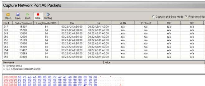
The **Capture Network Port A0/A1 Packets** function located on the **Menu Bar** allows you to capture packets flowing through **Network Port A0/A1**. NuSet-MiniTAP has two different modes available for capturing packets:
