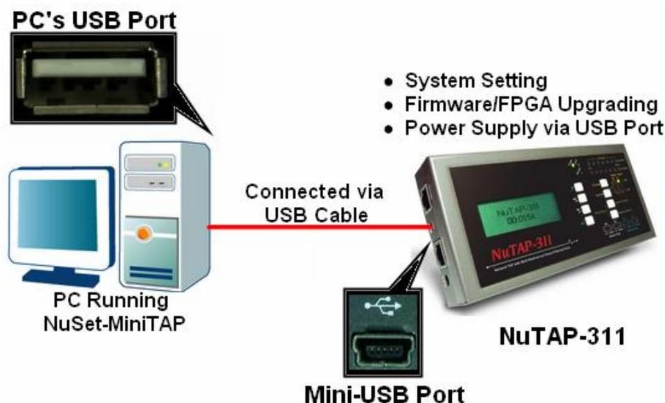
NuTAP-311 comes with GUI (Graphic User Interface) utility software **NuSet-MiniTAP** for setting test criteria and system management. Please note that you have to connect NuTAP-311 to your PC with a **USB** cable as shown in the figure above.
