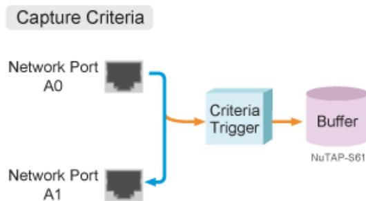
With **Capture Criteria**, transmitted packets from NuTAP-311's Network Port A0 to A1 (or the other way around) that meet the criteria set in Capture Criteria will be captured and stored in NuTAP-311's buffer memory. All packets captured and stored this way can be accessed via any Monitor Port upon user requests.
