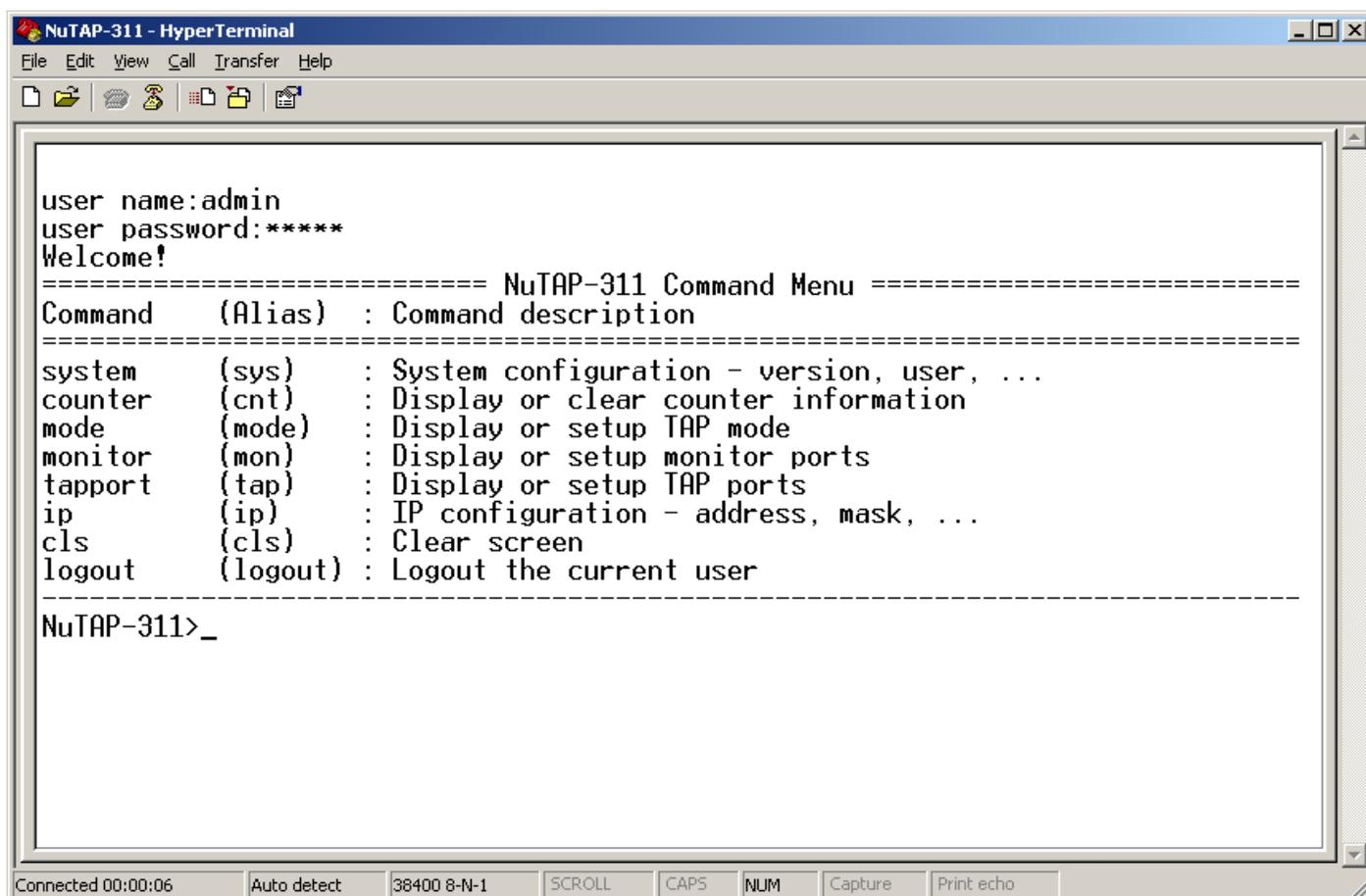
After logging in NuTAP-311 via HyperTerminal, a **NuTAP-311 Command Menu** will be displayed, showing NuTAP-311's HyperTerminal commands. Please see the table down below for brief descriptions of NuTAP-311 commands:
