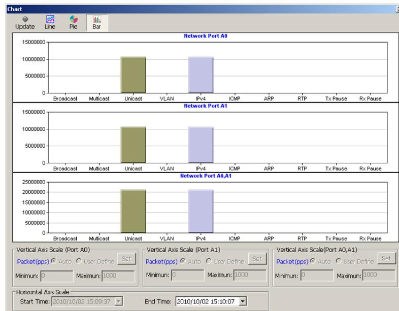
The **Bar Mode** displays **Network Port A0**, **Network Port A1**, and **Network Port A0/A1**'s statistics including: **Broadcast**, **Multicast**, **VLAN**, **IPv4**, **ICMP**, **ARP**, **RTP**, and **Tx/Rx Pause**.
