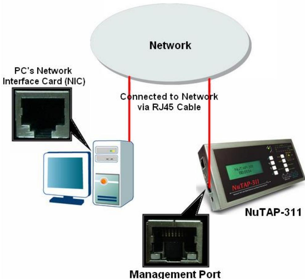
NuTAP-311 is embedded with a configuration webpage, and can be accessed by connecting NuTAP-311's **Management Port** to the network which your PC is connected to, as shown in the figure above.
