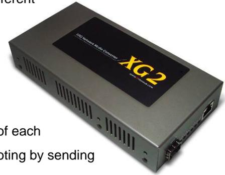
All XG2 Series are equipped with real-time LEDs which display the status of each port. The built-in loopback functions make XG2 Series ideal for troubleshooting by sending packets like BERT patterns to network equipment.
